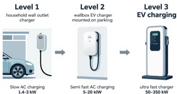
Fig. 1. Comparison of electric vehicle charging levels
