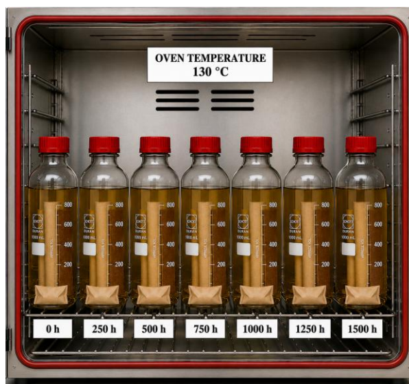
Fig. 1. Photograph of the dielectric liquid–solid insulation–metal catalyst systems placed in a temperature-controlled oven for the accelerated thermal ageing experiment.
