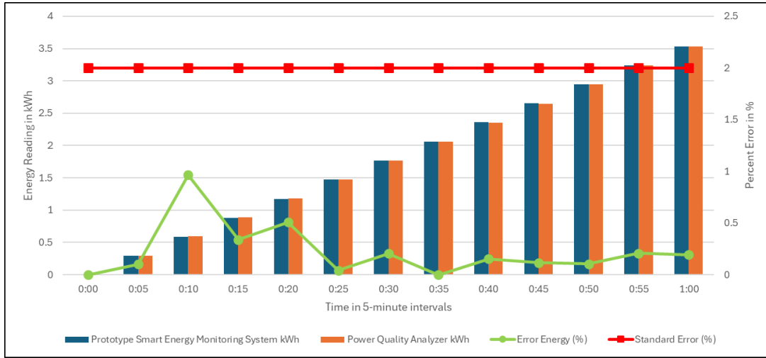
Fig. 9. Performance of the monitoring system in the total cumulative energy reading against the PQA in Scenario 1
