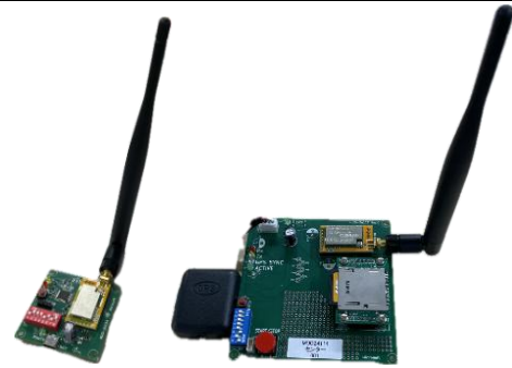
Fig.5. LoRa Transmitter Terminal (Left) / Aggregation Station (right).
