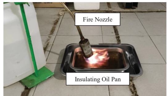
Fig. 2(b). The surface of the transformer insulating oil was blasted by the fire nozzle
