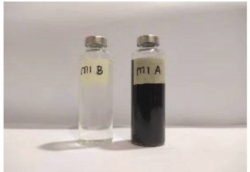
Fig. 3(d). Midel 7131 colour changes before & after the fire resistance tests
