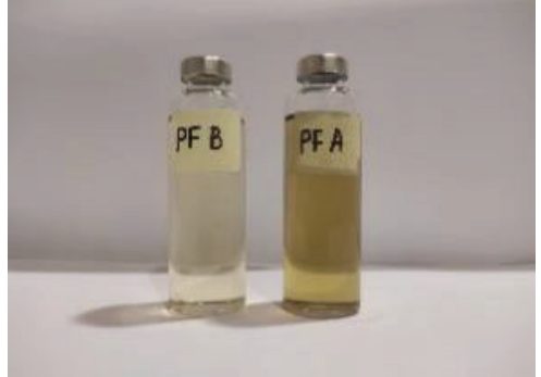
Fig. 3(c). Palm fatty acid ester colour changes before & after the fire resistance tests
