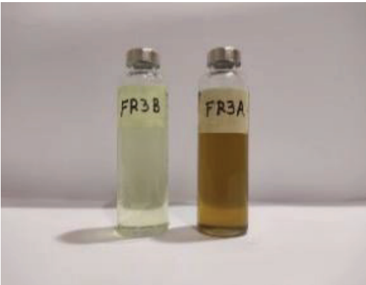
Fig. 3(b). FR3 colour changes before & after the fire resistance tests
