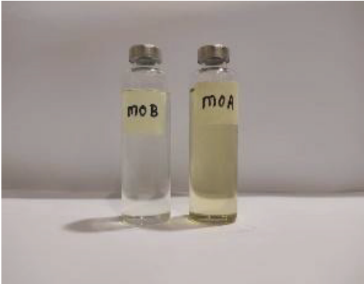
Fig. 3(a). Mineral oil colour changes before & after the fire resistance tests
