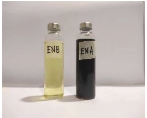
Fig. 3(e). Midel eN 1204 colour changes before & after the fire resistance tests
