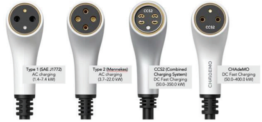
Fig. 2. Common electric vehicle charging connector types
