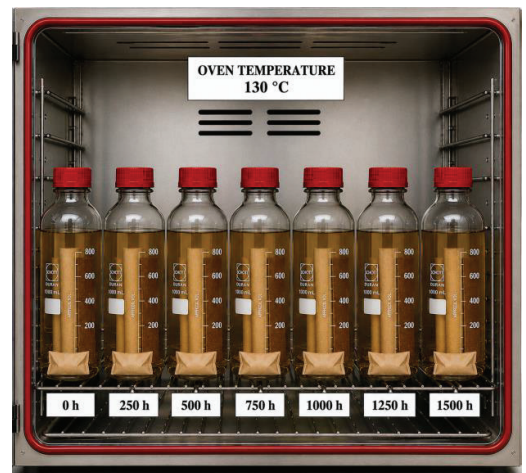
Fig. 1. Photograph of the dielectric liquid–solid insulation–metal catalyst systems placed in a temperature-controlled oven for the accelerated thermal ageing experiment.
