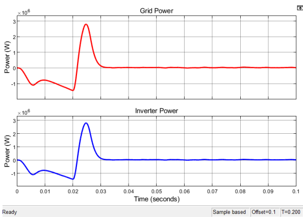
Fig. 14. Power for the Grid & Inverter
