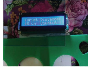
Fig 14. LCD display the distance and number of detected garments
