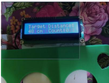
Fig 14. LCD display the distance and number of detected garments
