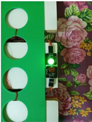
Fig 13. LED indicates the present of garment
