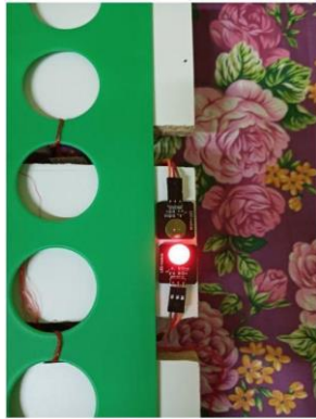
Fig 12. LED indicates the absence of garment
