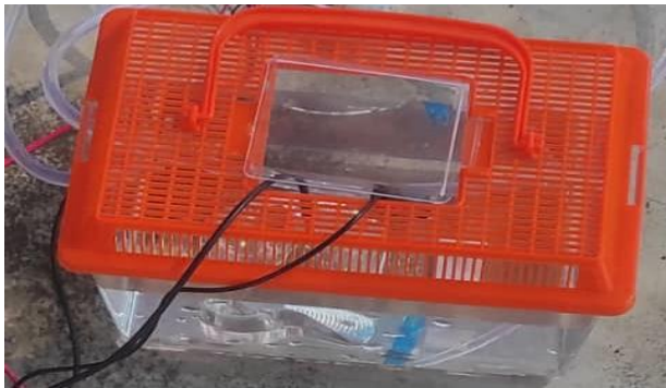
Fig. 8.prototype testing with a three-liter sample water tank.
