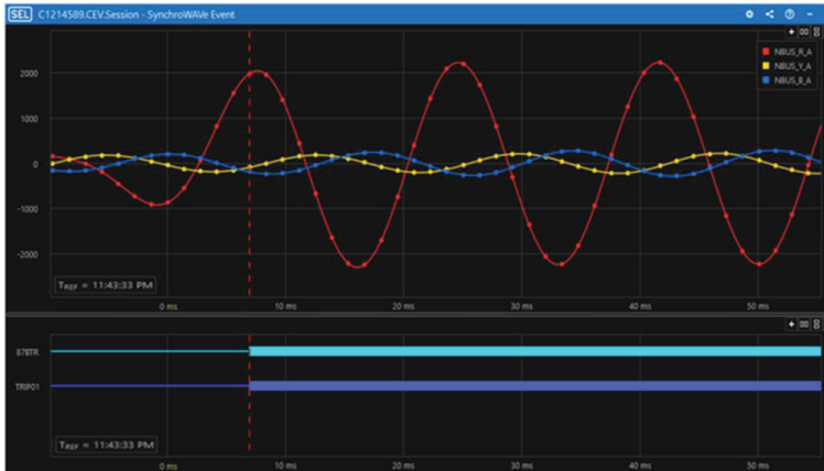
Fig.11. SEL-487B IED trips instantaneously
