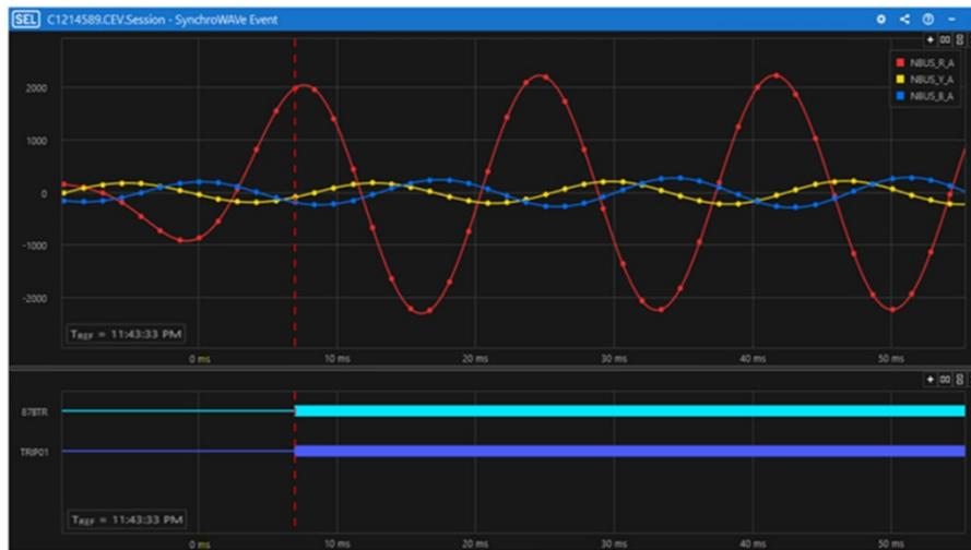
Fig.11. SEL-487B IED trips instantaneously
