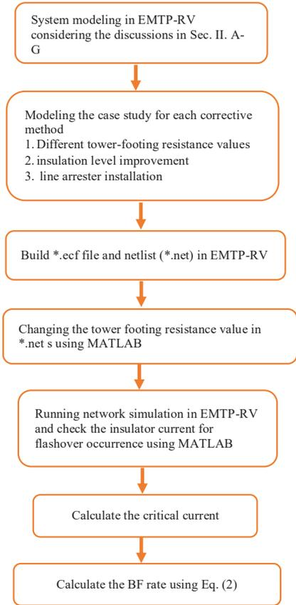
Fig. 5. Flowchart of the procedure used for calculating the BF rate
