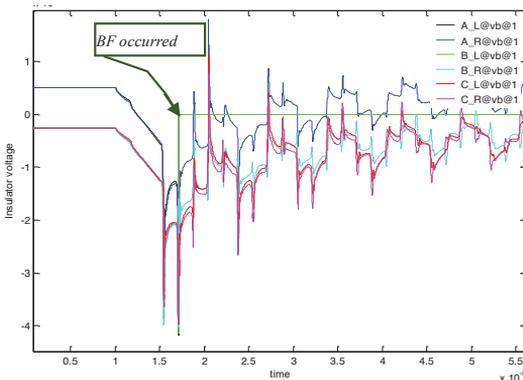
Fig. 7. Voltage across the insulator
