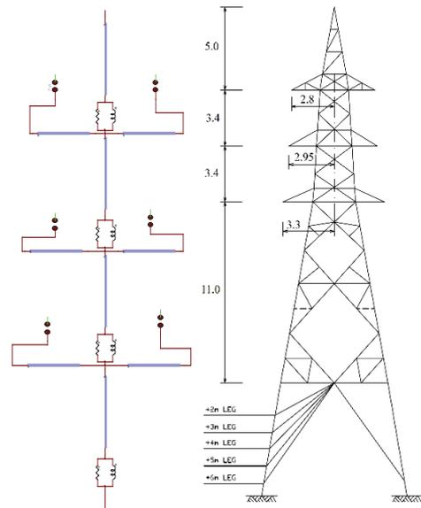
Fig.1. The tower dimensions and circuit model unit model
