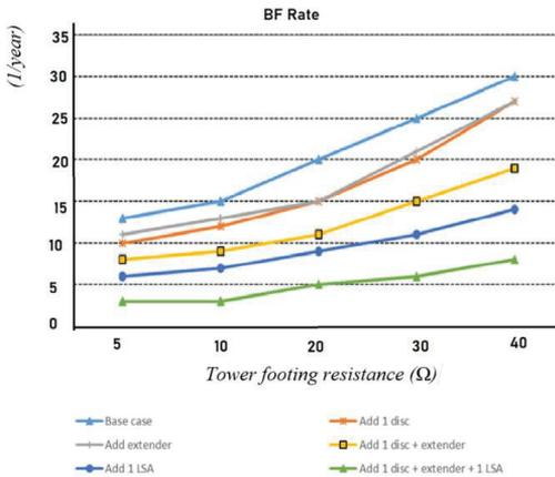
Fig. 6. BF rate calculation for different lightning protection methods
