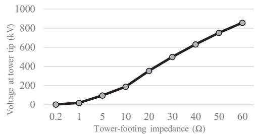
Fig. 4. The effect of the tower-footing impedance on the high voltage of the tower due to the lightning wave
