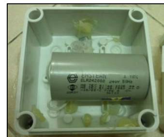
Fig. 4. Capacitor in another brand of ESD
