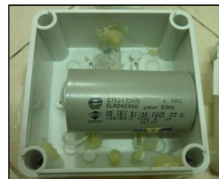
Fig. 4. Capacitor in another brand of ESD
