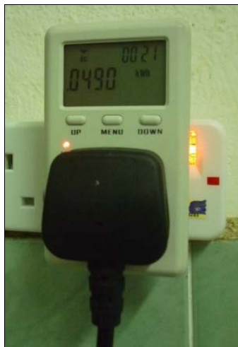
Fig. 6. Watt Meter WF-D02A plugged in socket between appliances
