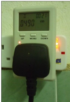
Fig. 6. Watt Meter WF-D02A plugged in socket between appliances
