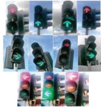
Fig. 3. Results of the traffic light arrow after the process of histogram equalization.
