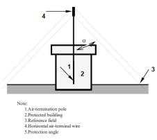
Fig. 5. Franklin method of lightning protection system [11].
