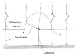
Fig. 3. Lines of a lightning tongue for a particular lightning current [11].
