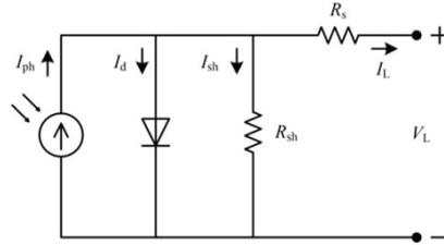
Fig. 1. Single Diode Model (SDM) [19].
