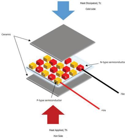
Fig.1. Schematic diagram of thermoelectric module
