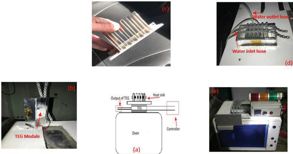
Fig. 2. Experiment Setup Diagram. (a) Block diagram; (b) Location of TEG Module; (c) Custom-made heatsink; (d) Water hose inlet and outlet; (e) Complete entire experiment setup
