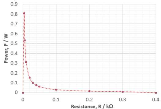
Fig. 6. Power output versus resistance
