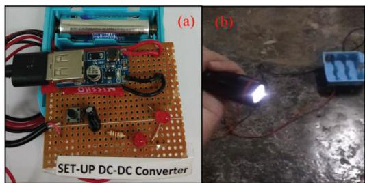
Fig. 8. (a) Fabricated boost up DC-DC converter; (b) Power-up the LED-torch light
