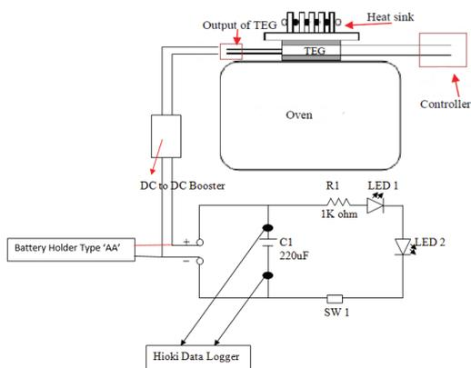
Fig. 7. Block Diagram of battery charger
