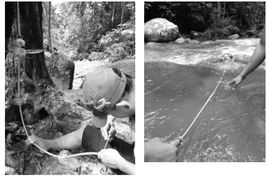
Fig. 4. The arrangement of the FMRCT on site
