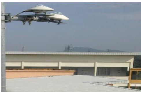
Fig. 4. CMP11 thermopile pyranometers with ISO 9060 Secondary Standard
