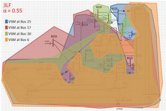
Figure 4: Area covered by the installed VSMs when voltage sag occur on the IEEE 30-bus system for 3LF fault and \alpha = 0.55 p.u.
