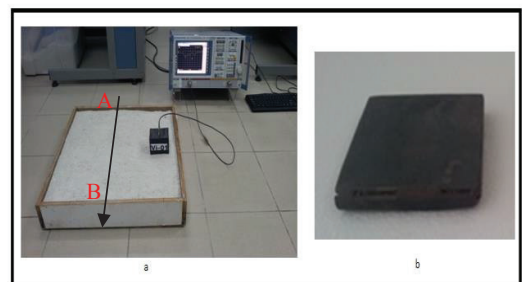
Fig. 12. The process of testing the GPR Hybrid system using a wooden chamber containing dry sand and iron object
