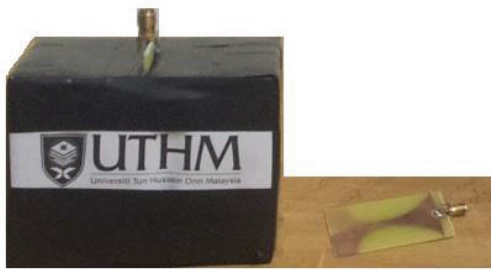
Fig. 9. Vivaldi antenna which has been fabricated and packaged
